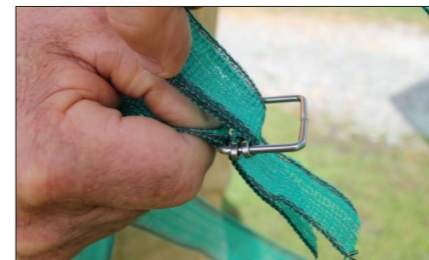
Slide both bars to the curved end of the joiner
