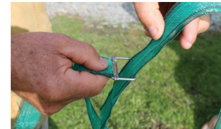
Pass both ends down through gap, about 20cm
