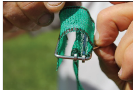
Push bars across from straight side and thread tape down
