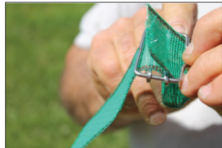
Push bar nearest to curved end across and thread tape up between bar and curve
