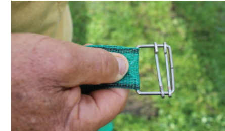
Thread one tape 500mm down through curved end and use tape to hold joiner
